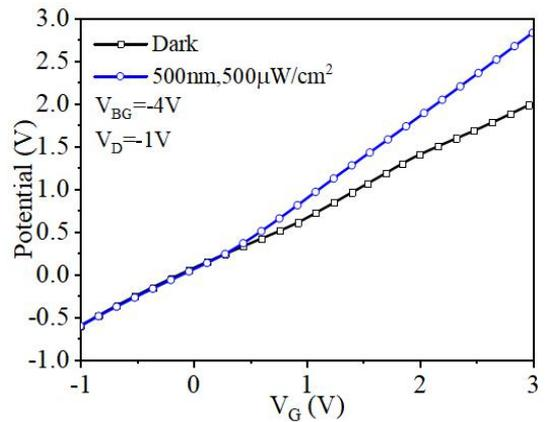
Figure 4: Comparison of potential in the dark and under illumination, extracted at the midpoint of  $MoS_2/HfO_2$  interface
