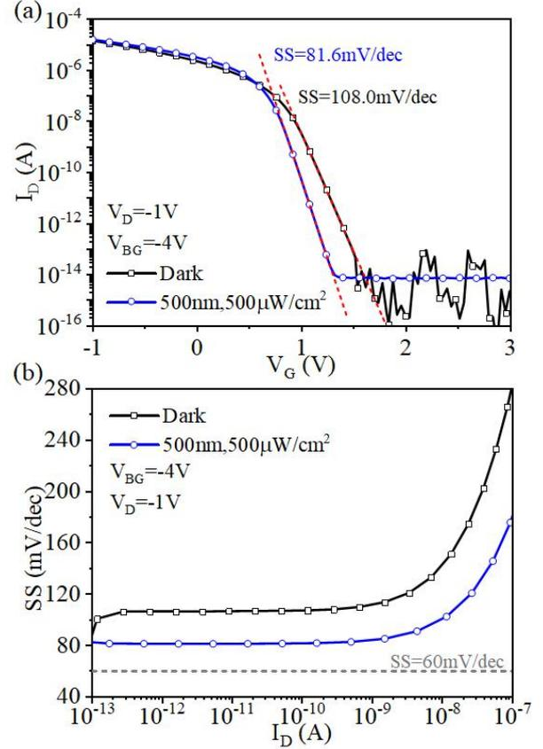
Figure 3: (a) Simulated  $I_D$ - $V_G$  curves in the dark and under illumination at  $V_D = -1V$  and  $V_{BG} = -4V$ ; (b) extracted SS versus  $I_D$
