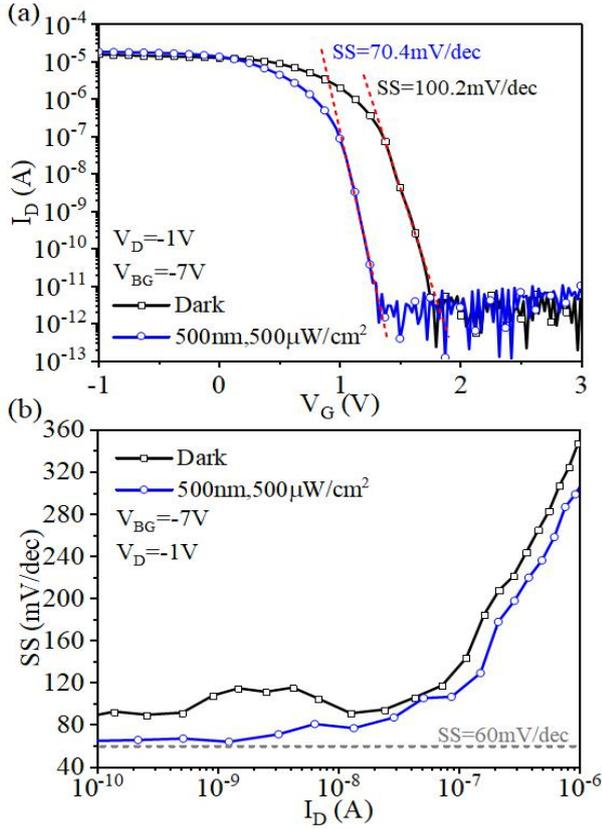
Figure 2: (a) Experimental  $I_D$ - $V_G$  curves in the dark and under illumination at  $V_D = -1V$  and  $V_{BG} = -7V$ ; (b) extracted SS versus  $I_D$
