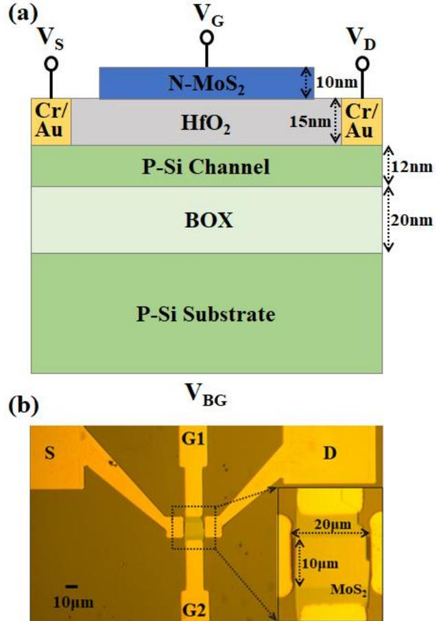
Figure 1: (a) Schematic view and (b) microscope image of the device
